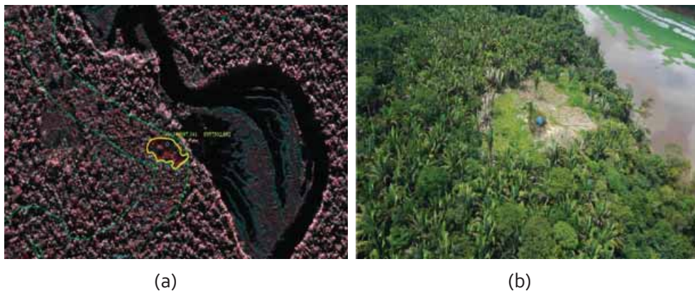
Figure 3. RGB composition of multitemporal SAR orthoimages showing a deforestation in the region delimited by the yellow contour (a) and corresponding aerial photograph of this deforested area (b).
